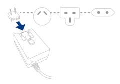
2. Connect the power supply to a wall outlet and to the drive.
