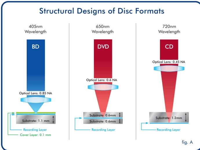
The LaCie d2 Blu-ray Drive uses a blue-violet laser and improved lens specifications (wavelength, NA-numerical aperture) allowing for a laser beam focus that’s approximately one-fifth smaller than the red laser used to burn DVDs.
