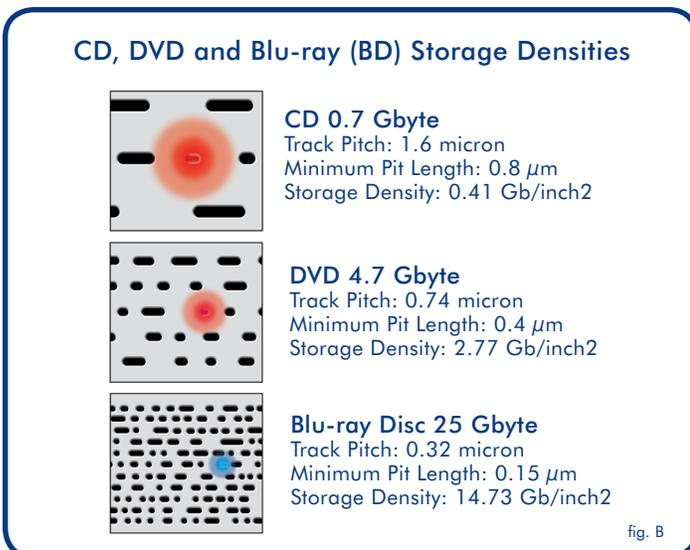
Also, because the disc’s first data layer is positioned at the very top of the disc structure, there is more space left underneath it for an additional layer, allowing for storage on 2 layers (50GB).
