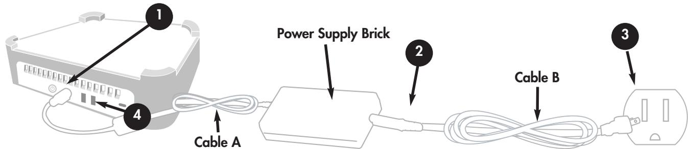
There are two cables that are supplied with the power supply: one cable (A) connects to a power outlet, such as a wall outlet or a surge protector; and the other cable (B) connects to the LaCie drive.
